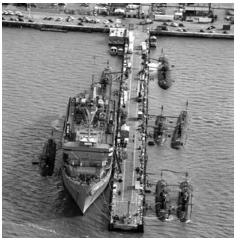
Submarine tenders are floating submarine supply and manufactory facilities. Prepositioned around the world, they can fix just about anything that goes wrong on a submarine.
