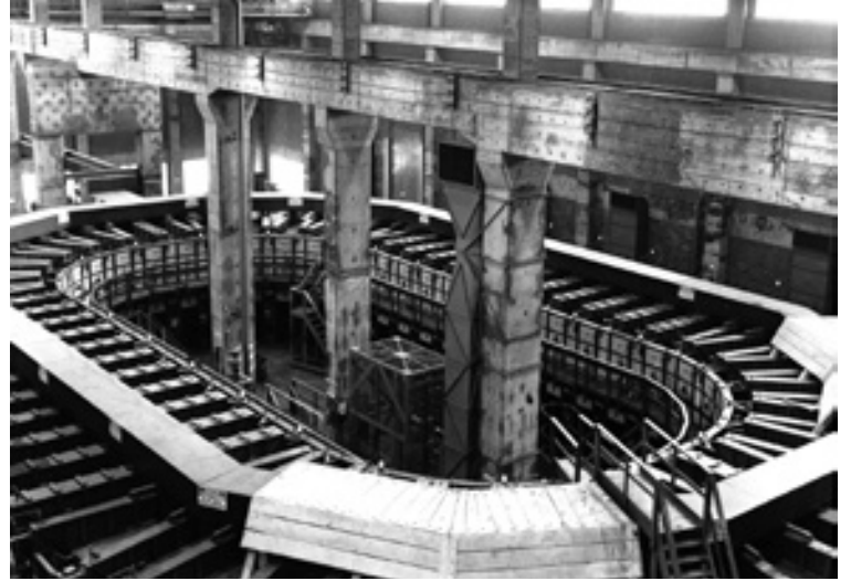
Calutron at the Y-12 Plant at Oak Ridge, from the Manhattan Project, used for uranium enrichment
