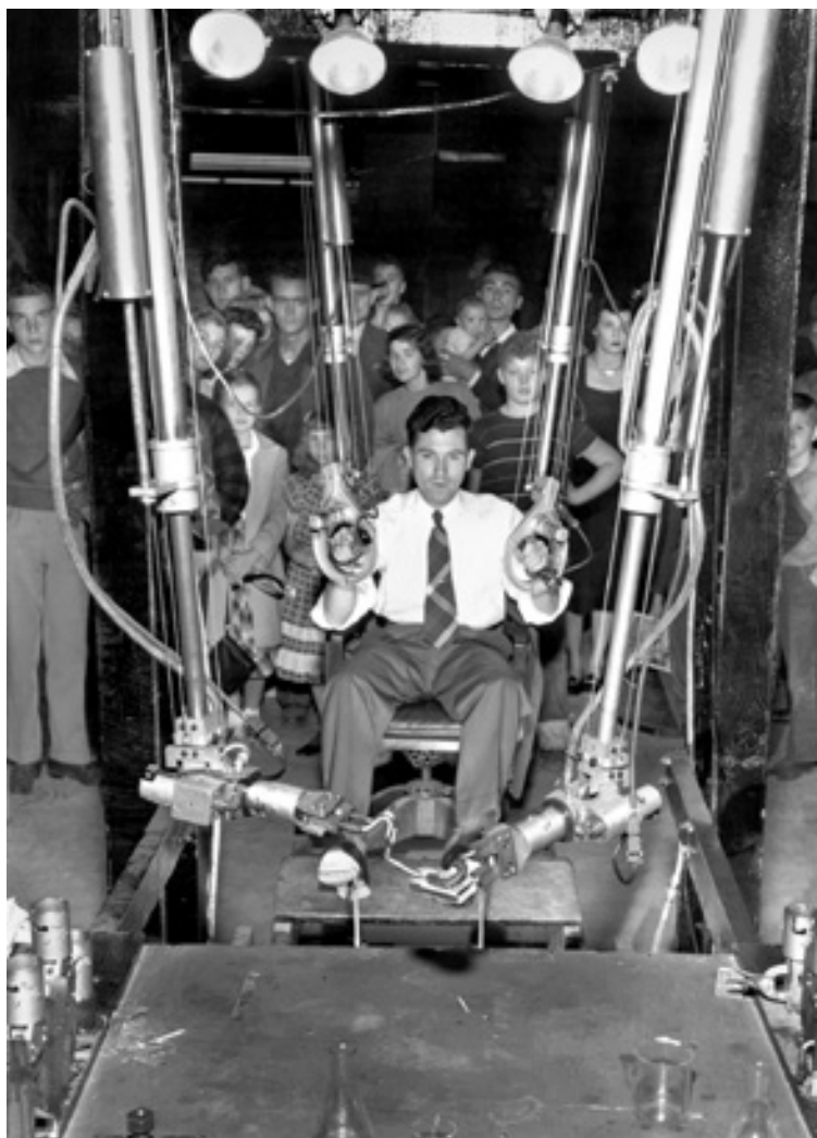
A 1949 exhibit in Oak Ridge showed the early use of "mechanical hands" for remote handling of atomic materials.
